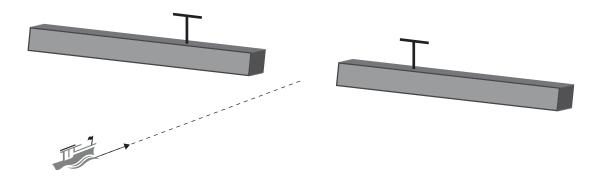
(f) If a boat travels along the central path, it receives a strong radio signal. If the boat moves to one side of the central path, the amplitude of the radio waves received **decreases**.
